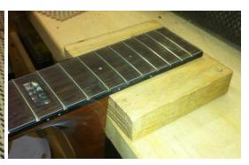
4) Trim any fret overhand/excess with the end nippers flush to the fingerboard.
