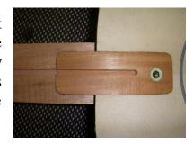
**High Tang/In Plane Note:** You will also need to be sure the bottom of the tang mortise is at the same height as the mortise in the body. If they are not equal, set up a router with a straight bit and freehand the groove staying away from the sides of the mortise. Clean up cut with a chisel. Typically, the body mortise would need to be lowered by a very small amount....1/32" to 1/16".
