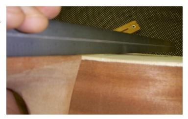
Next, you should place the fingerboard on top of the neck with the bridge in its rough location. Place the straight edge on top of the fingerboard and project it out to the bridge. *The straight edge should be above the height*
